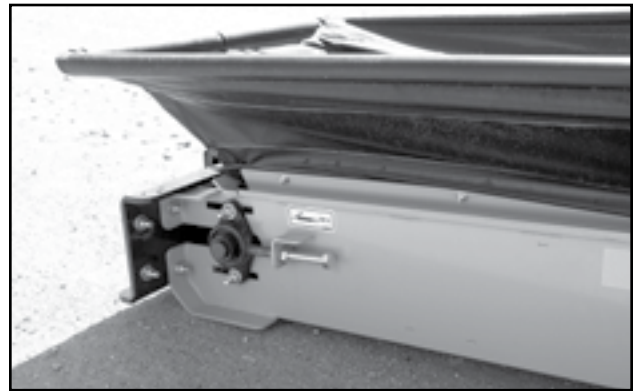
Fig 73 - Adjustment bolt at tail roller
