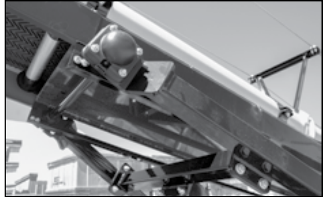
Fig 67 - Upper lift bearings
