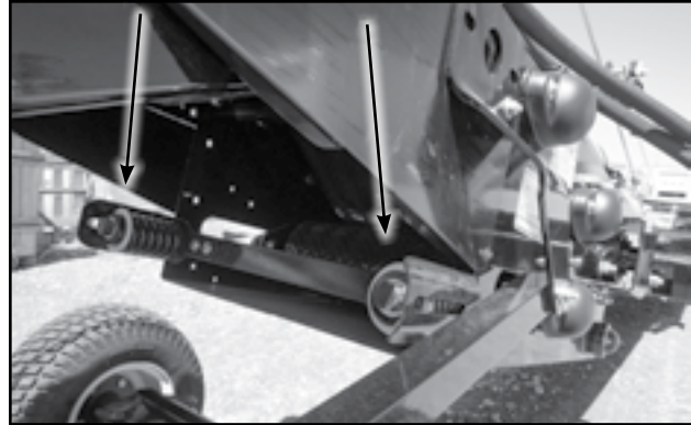
Fig 55 - Tension bolts, below drive box
