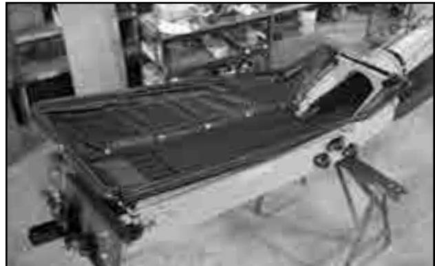
Fig 240 - Finished open transition hopper
