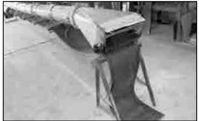
Fig 157 - Belt at discharge
