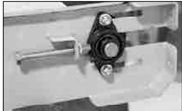
Fig 192 - Adjust bearing placement
