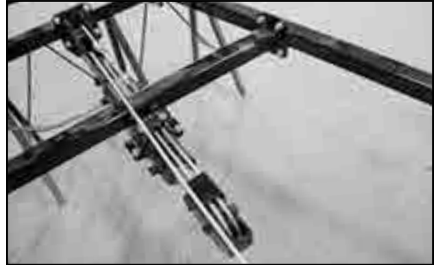
Fig 107 - Remove slack from lift cable
