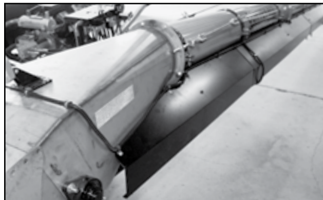
Fig 206 - Anchored undercarriage saddle
