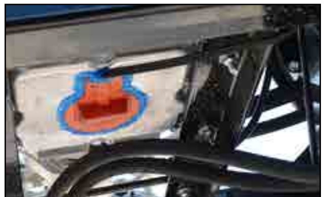
Fig 9 - 125 watt heater for engine
