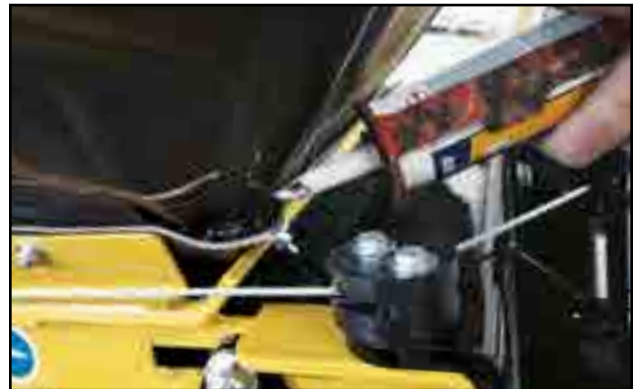
Fig 111 - Silicone gap in front corners
