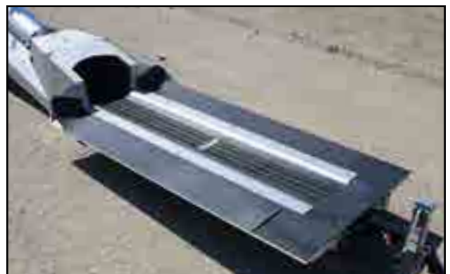
Fig 24 - Rail car hopper
