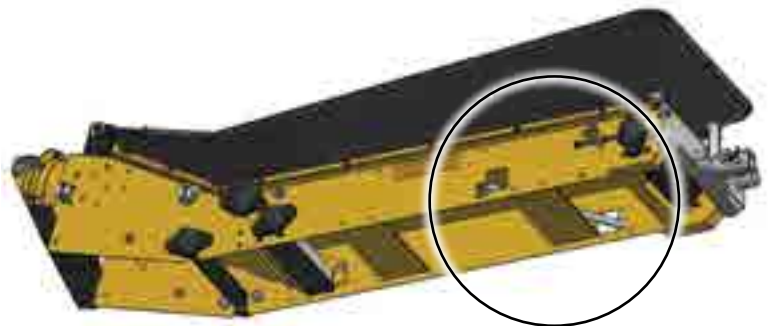
Fig 35 - Belt Scraper inside hopper frame
