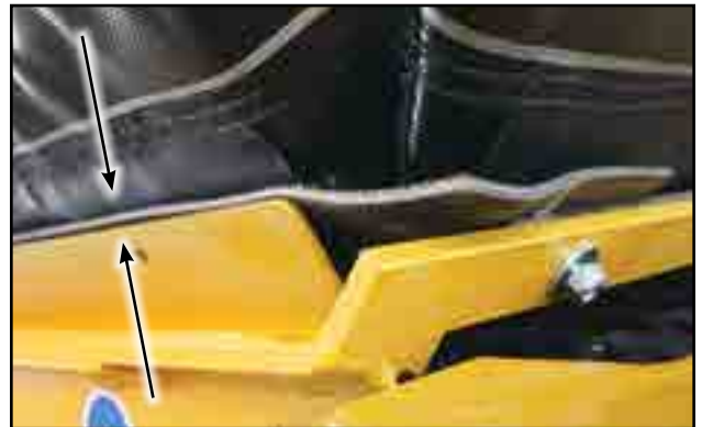
Fig 103 - Flashing flush with brackets
