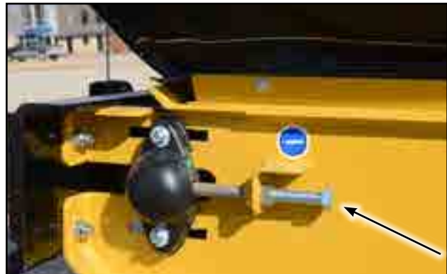
Fig 59 - Adjustment bolt on tail roller
