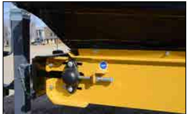
Fig 77 - Adjustment bolt at tail roller
