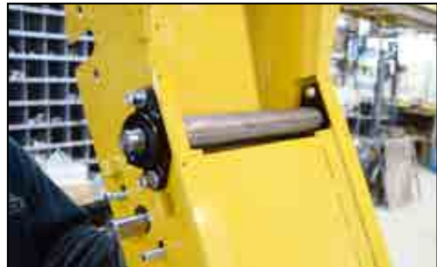
Fig 105 - Transition rollers with guide plates
