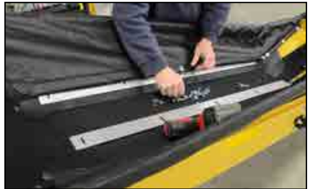
Fig 212 - Layer side flashing pieces
