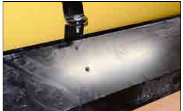
Fig 178 - Attach windguard to return roller bracket
