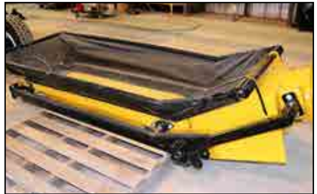
Fig 109 - Hopper frame, shown with canvas installed
