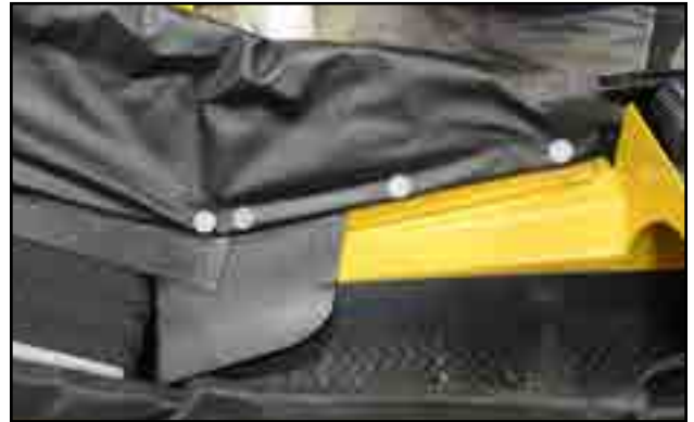
Fig 211 - Secure canvas and flashing to frame bracket
