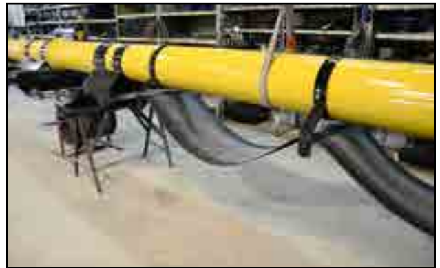
Fig 137 - Lay belt over return rollers
