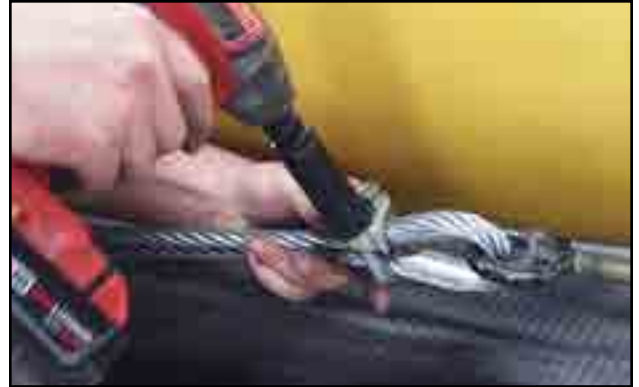
Fig 172 - Tighten discharge eye bolts
