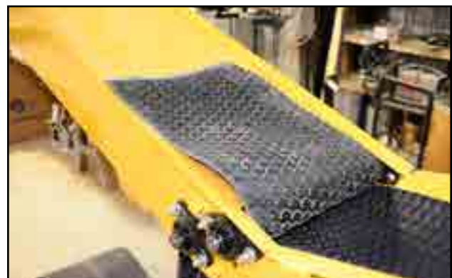
Fig 143 - Pull belt across hopper
