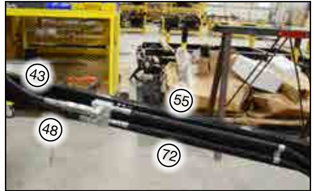
Fig 52 - Check valve hoses to lift cylinder
