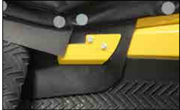
Fig 215 - Tighten bolts and install flashing clamp
