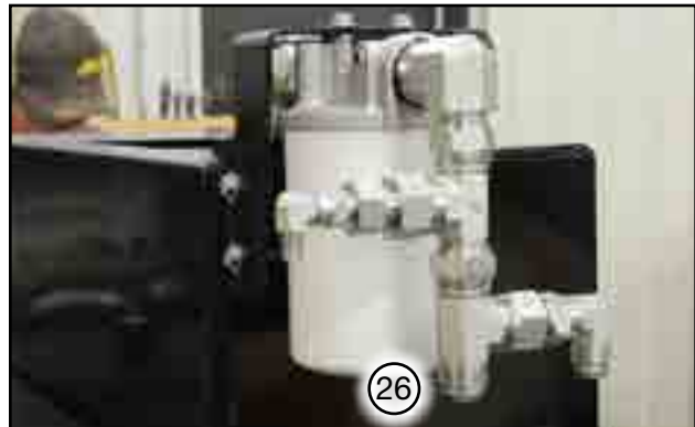
Fig 67 - Return fittings when oil cooling fan is installed
