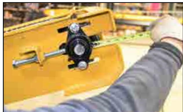
Fig 149 - Tighten hopper adjustment bolts
