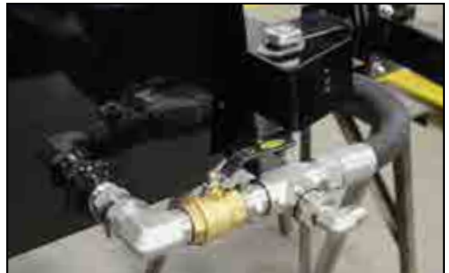
Fig 29 - Supply hoses if equipped with cooling fan
