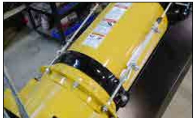
Fig 168 - Secure cable at hopper
