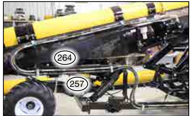
Fig 233 - Route hoses down driver-side arm
