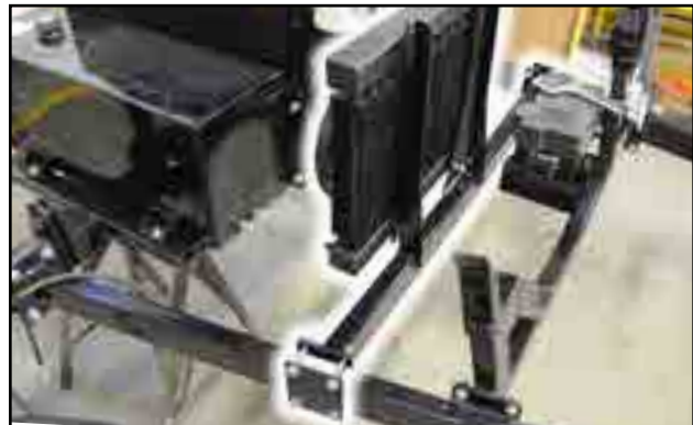
Fig 66 - Cross arm with hydraulic oil cooling fan
