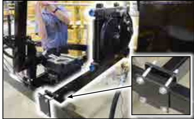
Fig 65 - Cross arm with hydraulic oil cooling fan
