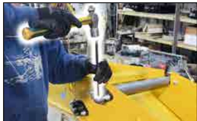
Fig 107 - Tighten Eccentric Locking Ring
