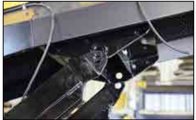
Fig 226 - Position rear arms of undercarriage to tube
