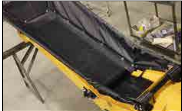
Fig 216 - Tighten bolts and install flashing clamp
