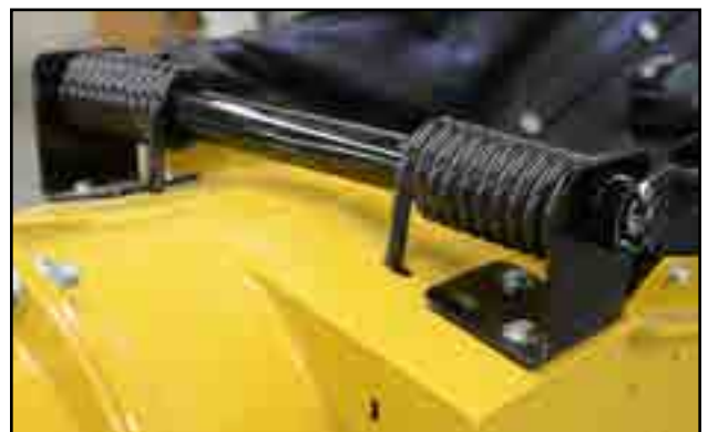
Fig 198 - Springs inside hopper hoop mount bar
