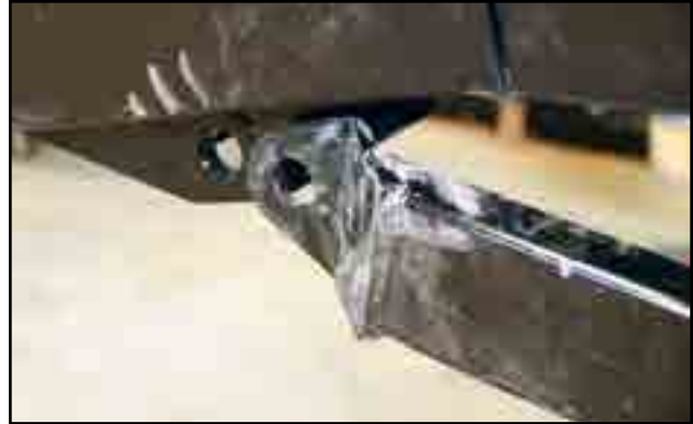
Fig 229 - Position front arms to undercarriage mount
