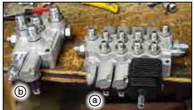
Fig 45 - (a) BM40/SD5/4 - Mover kit valve (b) BM70/SD11/1 - Conveyor belt valve
