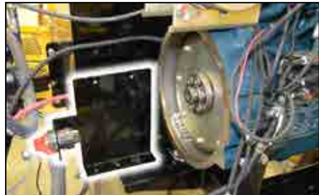
Fig 8 - Power shut-off switch mounted on plate
