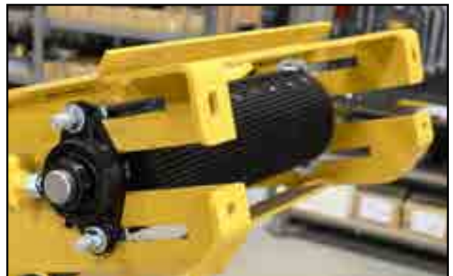
Fig 103 - Idler roller with bearings
