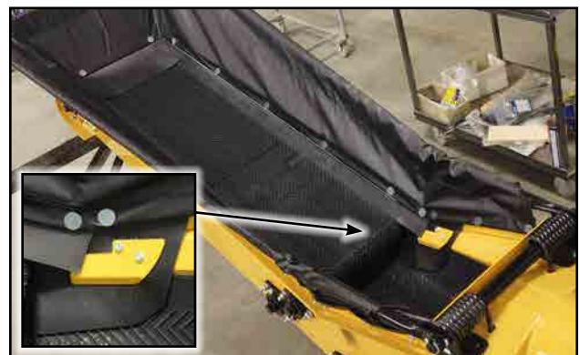
Fig 7 - Tighten bolts and install flashing clamp
