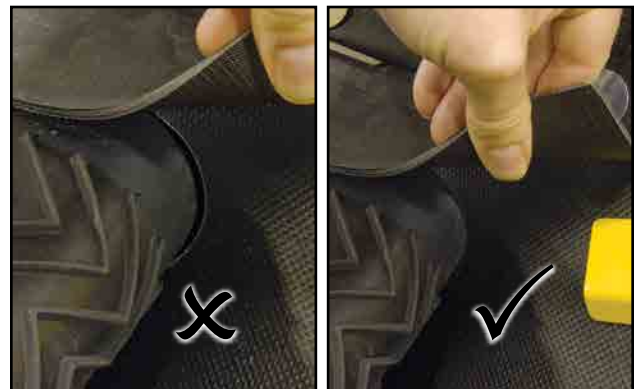
Fig 6 - Corner flashing must fit tight around the belt
