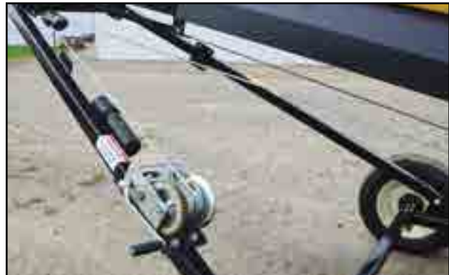
Fig 17 - Tube lift winch
