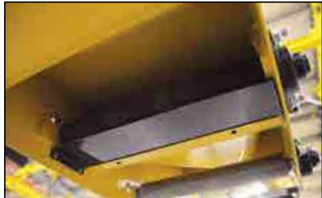
Fig 104 - Containment plate in place
