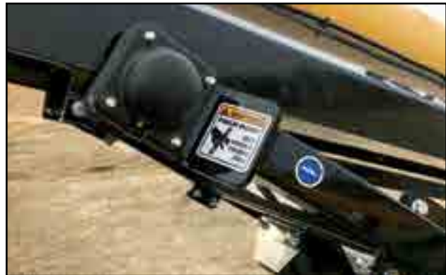
Fig 83 - Upper Lift Bearings
