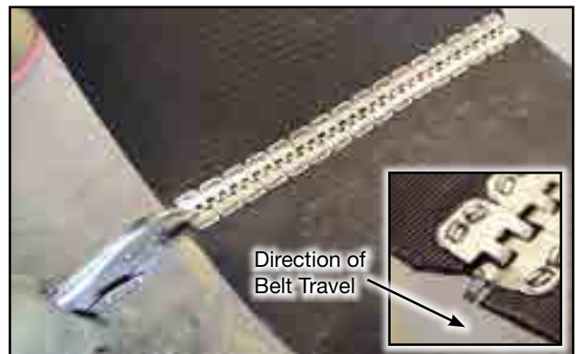
Fig 102 - Crimp lacing and taper belt corners
