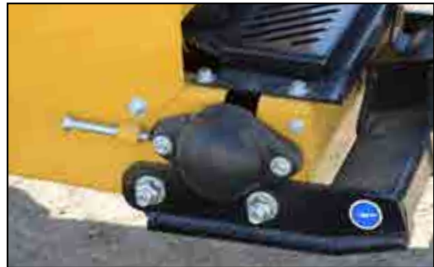
Fig 94 - Hopper idler roller bearing
