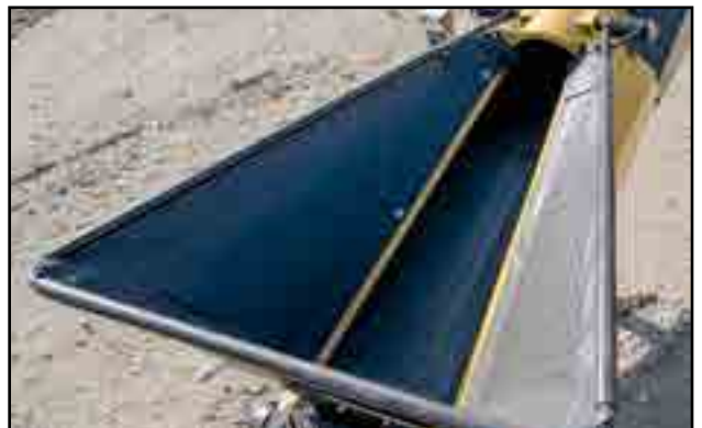
Fig 109 - Completed hopper with belt
