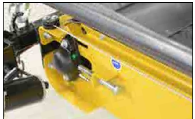
Fig 93 - Swing-out idler roller bearing
