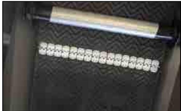
Fig 69 - Belt lacing and roller
