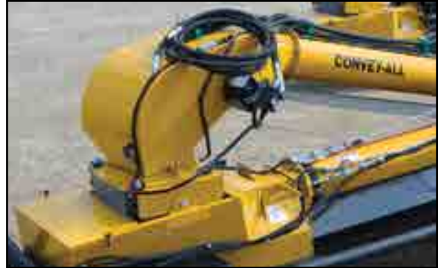
Fig 40 - Swing-out discharge to main conveyor hopper
