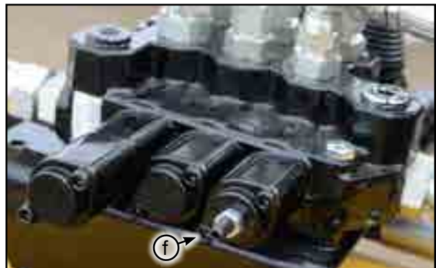
Fig 47 - Valve adjustment, rear of bank
