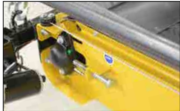
Fig 99 - Idler roller bearing on the swing-out
