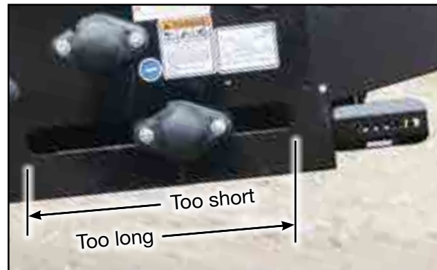
Fig 90 - "Slack Eliminator" roller. Belt length indication
