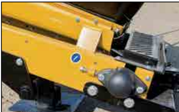
Fig 89 - Idler roller adjustment bolt
