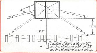
You can fill most planters with only one set-up. Conveyor can be transported to the front or rear.
