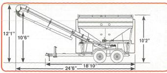
With a hopper height of 10' the BTS290 easily fits under most bulk seed loading stations. Easily reached with most front end loaders and forklifts. Ideal for farmers who use tote bags or seed boxes.
