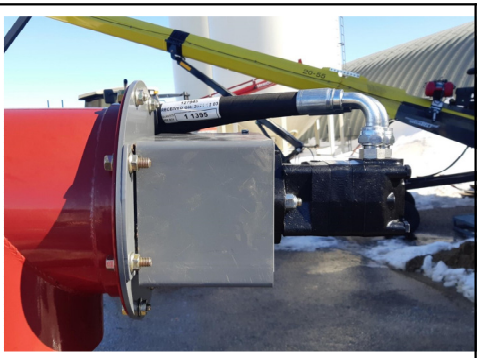
HEAD - END HYDRAULIC DRIVE ONLY
