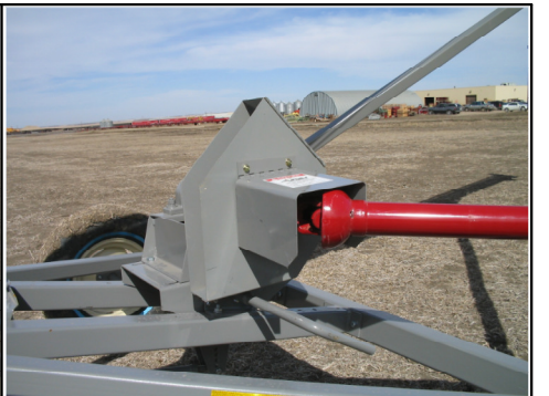
PTO ATTACHMENT GUARD BELT DRIVE ONLY
